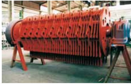
Rotor with bearings and V-belt pulley.
